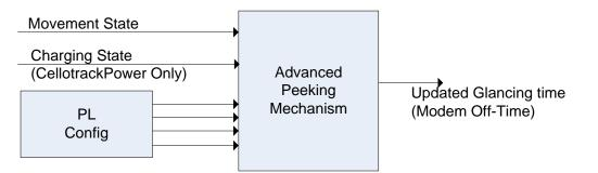
The following table describes the relations between the system state (Charging or moving) and the glancing time. Each system state glancing-time is represented by a dedicated configuration parameter. The unit's firmware will select the relevant configuration parameter when the system will change its state. The new glancing-time will be used in the next glancing period or if distress or Active Logged event will be triggered.
