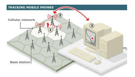
Positioning software performs a triangulation calculation on the information and the data is converted into a geographical location: strongest reception signal theoretically defines closest cells.
