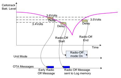
Early radio off message will be generated by the unit when the battery voltage reaches 3.6 Volts or below for 30 consecutive seconds. The early Radio off message will inform the server side that the unit's battery voltage is very low and that Radio off mode is about to start soon.
