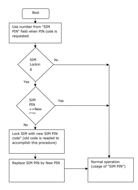
**NOTE**: Since the unit is actively modifying content of its programming cells (replacing the old Pin code by the new one) the configuration file and the actual content of programming will lose synchronization. It is very important to synchronize them by uploading the actual content of the configuration memory from the unit before next configuration cycle.
