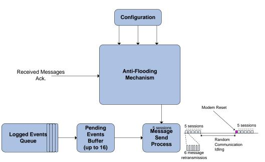
The block diagram above describes the Anti-Flooding mechanism. The Anti-Flooding mechanism's most important input is the received server acknowledgment; in case there are no acknowledge messages returned from the server, the Anti-Flooding mechanism will implement the following retry patterns:
