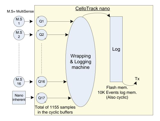
Each source has its separated state machine, and each buffer includes records and header.
