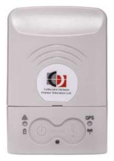
Each press on a Nano button when the unit is active activates a short audible beep by the buzzer (if enabled accordingly; read more about this setting <u>here</u>).
