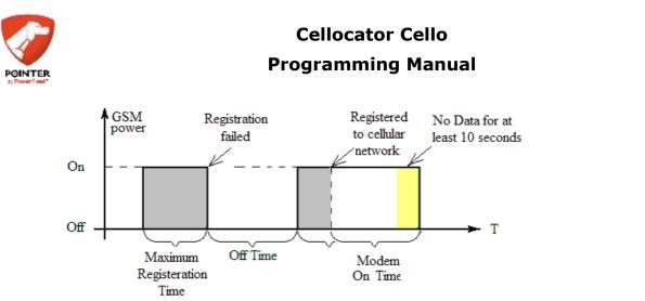
**Maximum Network Registration Time**: This parameter defines time interval, given to GSM modem for registration into cellular network. If registration wasn't accomplished during that time – the modem is being turned off for Off Time.
