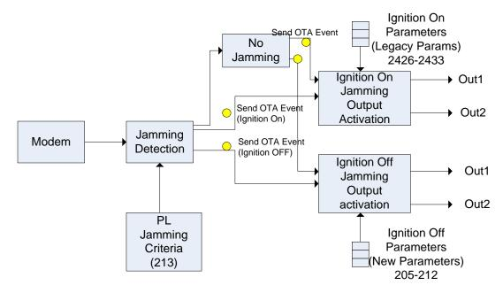
The following responses to jamming detection are available and switchable by unit's programming:
