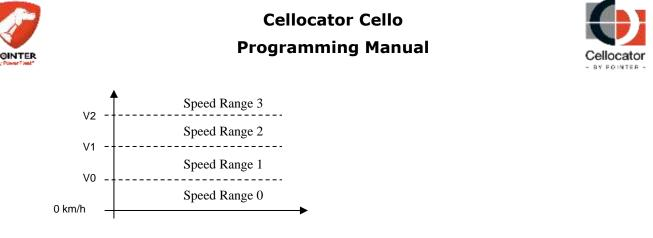
The speed ranges threshold (V0, V1, V2) must meet the condition: V0<V1<V2
